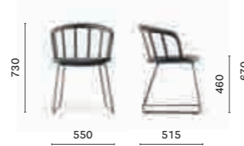
2855 Ash wood armchair, steel rod sled frame
