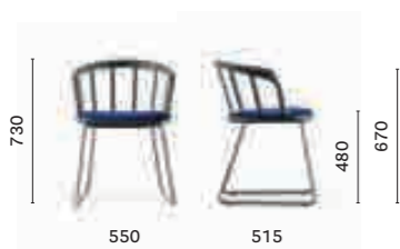
2856 Ash wood side chair, upholstered seat, steel rod sled frame
