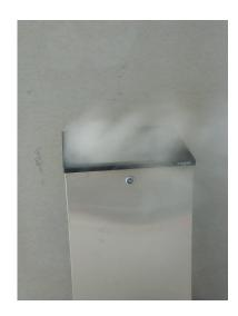
Design of the aperture clearly prevents intense fire inside the bin. Fire did not cause notable structural changes on the bin and structural tolerance of the fire load is excellent.
