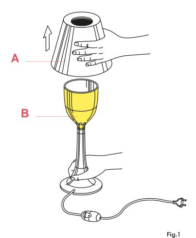
Remove the external diffuser (A) from the internal diffuser (B).
