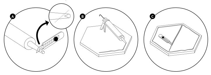
**ATTENTION!** Avoid staining the surface of the panel with the adhesive. Should you get some glue on the panel gently remove it with the tip of the carpet knife or a sponge. Do not smear the glue! Do not allow for the adhesive to dry – scraping it off may damage the panel surface. It is not recommended to glue the panels to one another.
