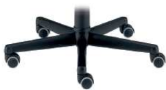
APN 5 star base with steel inner frame 25x30 mm th.2 mm Ø 670 mm, cover in black polypropylene. (Ansi-Bifma X5.1-1993/8)
