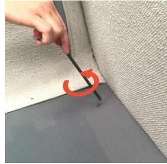
Loosen two hidden nuts in base as shown. Soltar los pasadores de la base.
